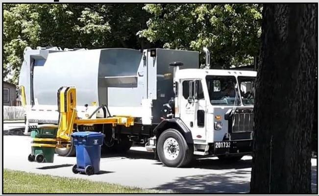
The KANN Automated Two Compartment Split Side Loader comes in several body sizes ranging from 20 to 28 cubic yards, has an arm reach of up to 10 feet, a loading cycle of 8 seconds and is capable of payloads up to 850 lbs./yd³.
