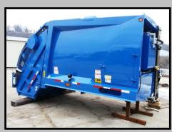
The Kann Rear Loader is designed so it can easily be shipped loose and mounted on a chassis at the customers' location.
