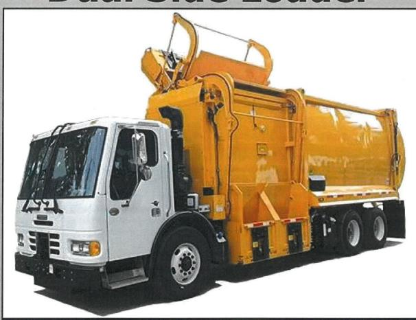
The KANN Curb Master Series Kann Pack Side Loader (Model KP) is a high capacity two compartment compacting unit with dual or single semi-automated side loading and easy tip-to-dump unloading.
