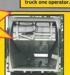
The KANN CoCollector has two independent volume adjustable compartments, split horizontally, that eliminates cross contamination between commodities
